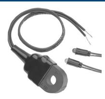
The LCS10T12 connected to the LPM12 or LPMG12 indicator is a low cost, easy to use, go/no-go indication system for the remote monitoring of current flow. The LCS10T12 is installed on an adequately insulated wire of the monitored load. Its 12in. (30.4cm) leads are connected to the LPM12 or LPMG12 panel mount indicator directly or via customer supplied wires up to 500 feet (152.4m) long.
