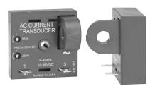
The TCSA Series is a loop-powered, linear output current transducer that provides an output that is directly proportional to the RMS AC current passing through the onboard toroid. The TCSA provides a 4 - 20mA output over a power supply range of 10 - 30VDC. Each unit is factory calibrated for monitoring in one of four ranges; 0-5, 0-10, 0-20, or 0-50A. The 0 - 5A range allows the use of external current transformers so loads up to 1200AC amps can be monitored.
