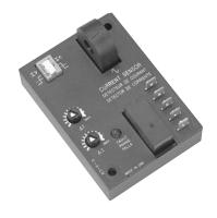
The ECS Series of single-phase AC current sensors is a universal, overcurrent or undercurrent sensing control. Its built-in toroidal sensor eliminates the inconvenience of installing a stand-alone current transformer. Includes onboard adjustments for current sensing mode, trip point, and trip delay. Detects over or undercurrent events like; locked rotor, loss of load, an open heater or lamp load, or proves an operation is taking place or has ended.
